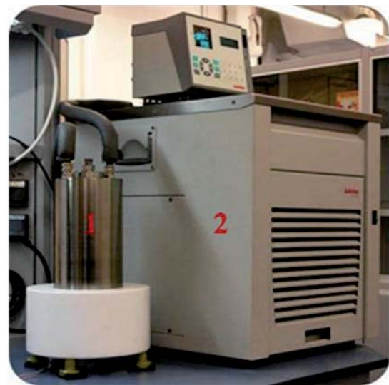
Figure 9: General view of the cell for thermal properties of fluids measurements under high temperature and pressure: 1 – hastelloy cell with the fluid under study coupled with heating/cooling annulus, and 2 - thermostatic unit.
