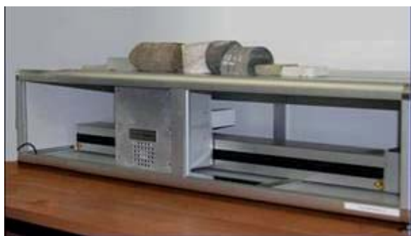
Figure 2: Optical scanning instrument for rock thermal property measurements on full cores.
