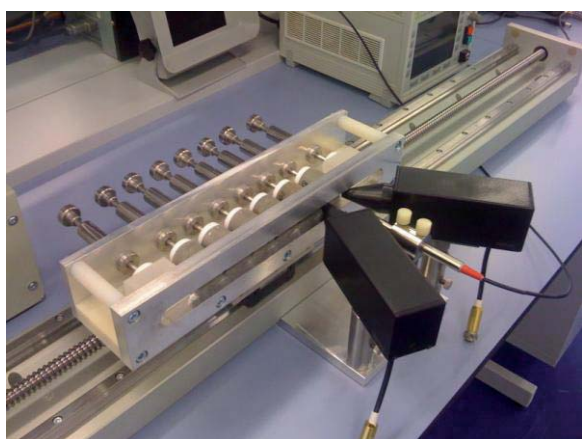
Figure 4: Laser optical scanning instrument for rock thermal property measurements on core plugs.
